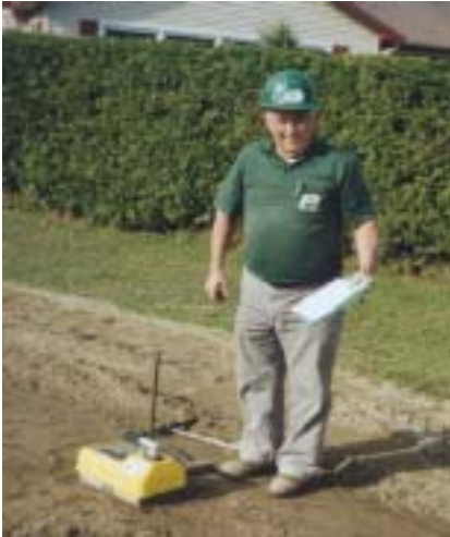
Leigh LaRock of Construction Materials Testing, Inc. Checks Compaction
