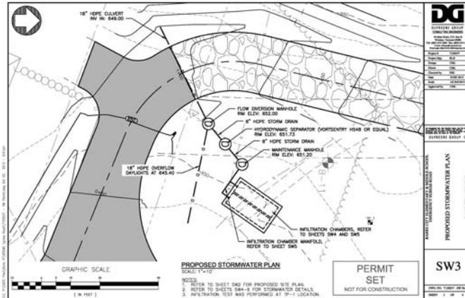
Dufresne Group provided the site and stormwater design for an emergency egress road at the Barre City Elementary and Middle School. The project consisted of a 1,075 linear foot access road and required stormwater treatment due to expansion of impervious area for a previously permitted parcel.
