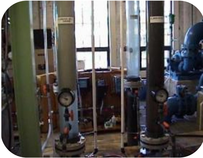
Parallel Process Comparison for Adsorber Clarifiers Followed by Mixed Media Filters (on right) Compared to Ozone Plus Coagulants (on left)
