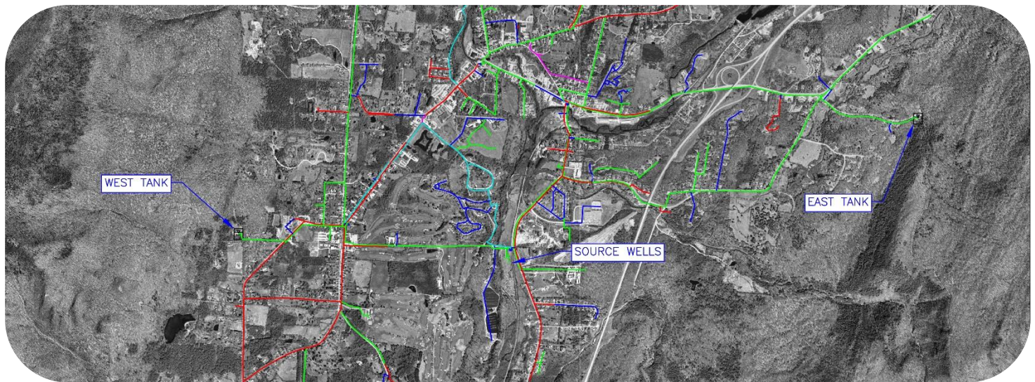
Map of Water System with Color-Coded C-Values
